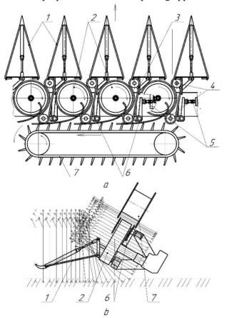
Fig. 1. **Disc-belt flax pulling apparatus:** 1 – dividers; 2 – pulling discs; 3 – pulling belts; 4 – rollers; 5 – spring–loaded fasteners; 6 – guide bars; 7 – transverse conveyor; a – top view; b – side view
