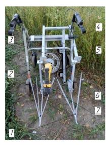
Fig. 2. Photo of the experimental setup: 1 – dividers; 2 – cart; 3 – pulling disk; 4 – pulling belt; 5 – rollers; 6 – centering clutch; 7 – cordless perforator
